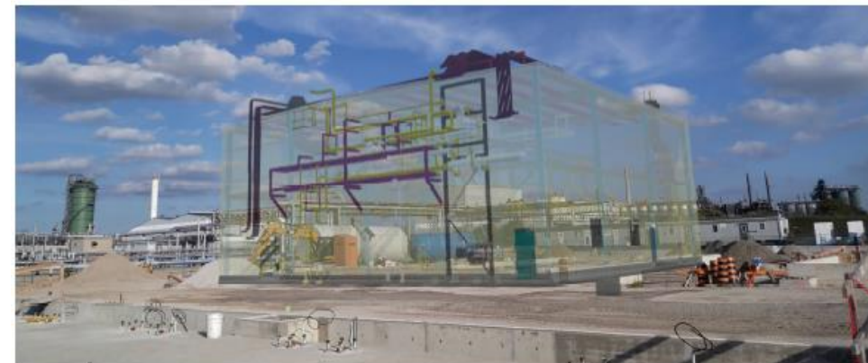
Future: 3-D Model Hologram Projection of Process Building, Which Will House Horizontal Modules (Not Shown) and Additional Equipment
