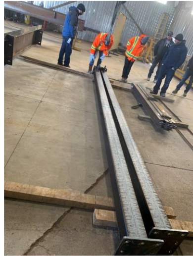
Finished steel verticals
