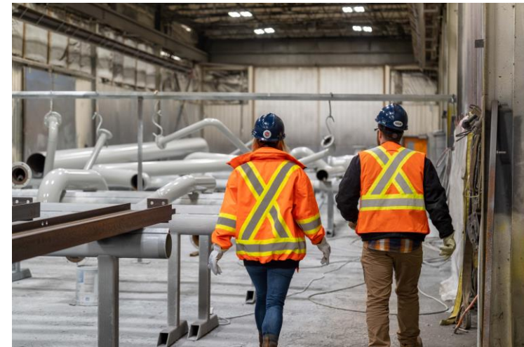
Painted pipe, including 80-foot pieces. Next, the pipes are assembled into pipe rack modules and shipped to the Origin 1 site for installation in the field
