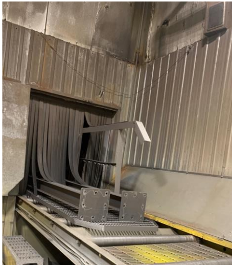
Blast cleaning steel verticals
