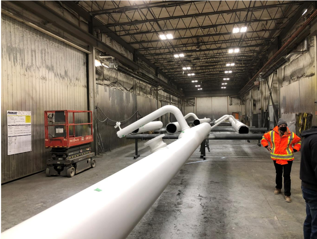
Painted pipe, including 80-foot pieces. Next, the pipes are assembled into pipe rack modules and shipped to the Origin 1 site for installation in the field
