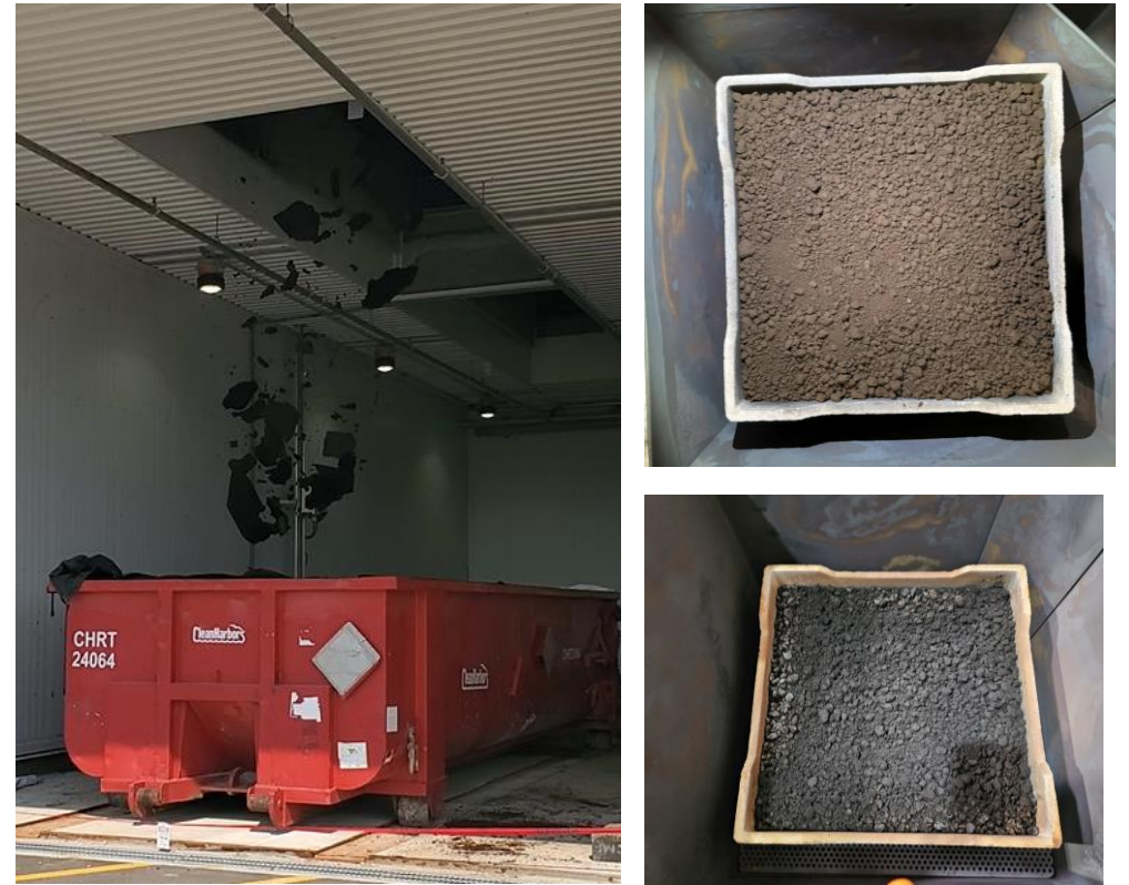
HTC shown dropping from the filter press at Origin 1 to roll off bin. Raw and carbonized HTC shown at right.
