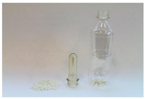
Advanced co-polyester made by Origin Materials and Husky Technologies using PET/F. Resin, mold, and bottle shown. (Photo: Business Wire)
